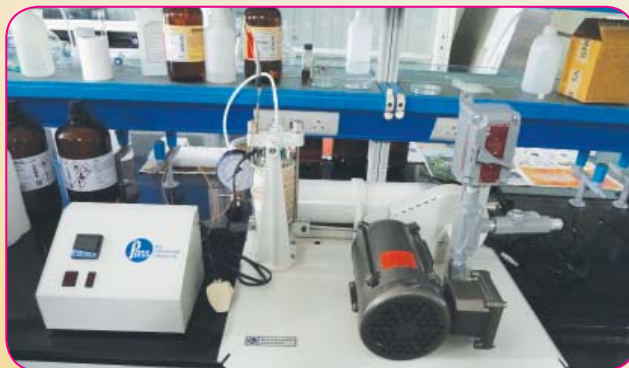
Newly installed Hydrogenation Apparatus at GBP
